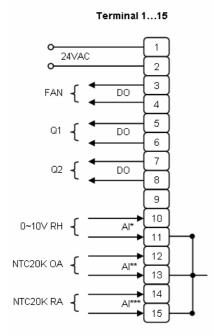
Al\*: 4~20mA or 0~10V (Humidity) AI\*\*: 4~20mA or NTC20K (Outside Air) AI\*\*\*: 4~20mA or NTC20K (Return Air)
